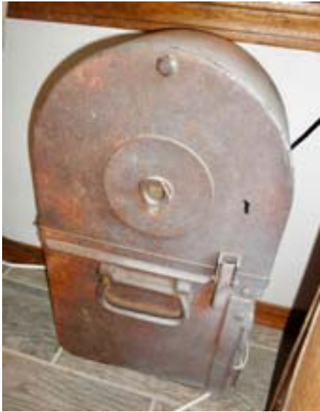
200-Round Tombstone Magazine for each .50 Caliber Browning Machine Gun
